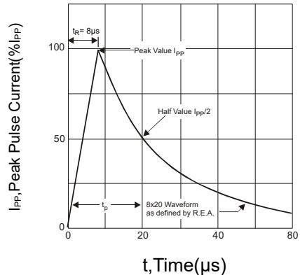
Figure 1: Typical 8 x 20µs Pulse Waveform
