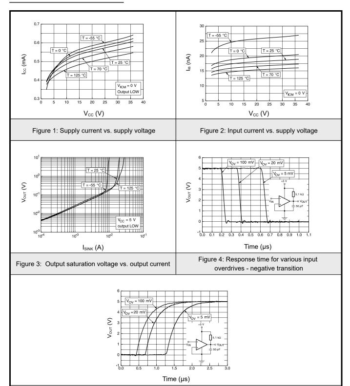
Figure 5: Response time for various input overdrives - positive transition
