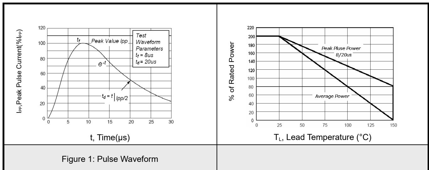
Figure 1: Pulse Waveform
