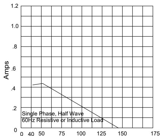
Average Forward Rectified Current - Amperes versus
