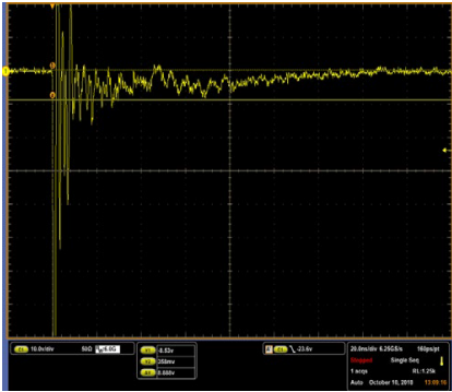
Figure 18: AQHV36 -8kV Contact ESD Clamping Voltage
