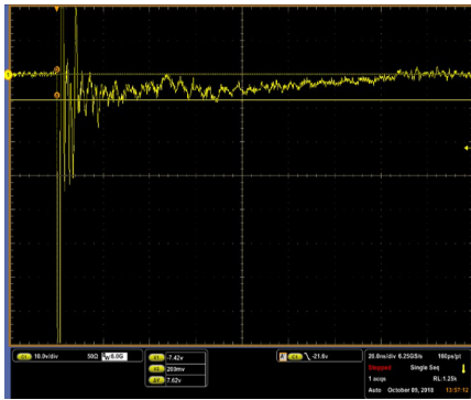
Figure 16: AQHV24 -8kV Contact ESD Clamping Voltage
