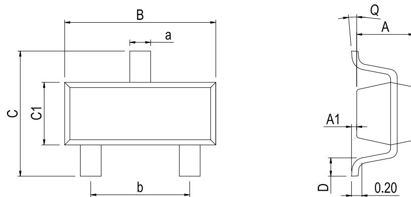
Dimensions In Millimeters(SOT-23)
