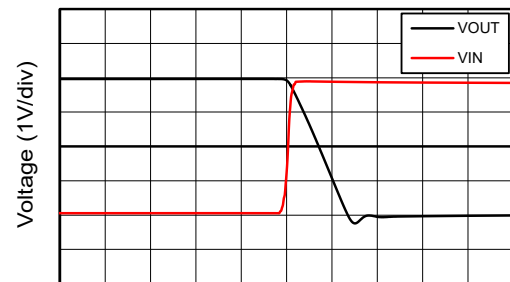
Time (500 ns/div), Falling output
