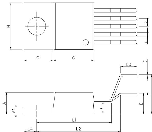
**Dimensions In Millimeters(TO220B-5)**
