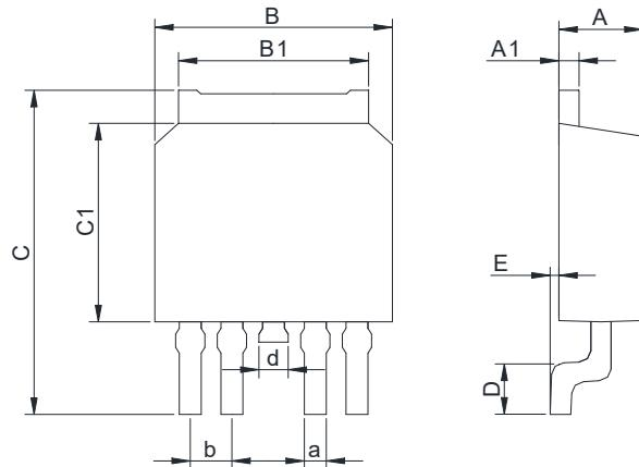
**Dimensions In Millimeters(TO-252-4)**
