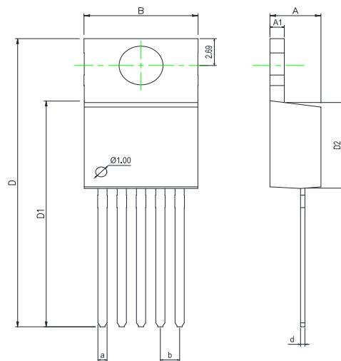
Dimensions In Millimeters(TO-220-5)
