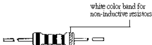
4.2.4.2 Marking: Marking is made on the surface with Rated Wattage, Nominal Resistance, Tolerance, and "NON-IND".
