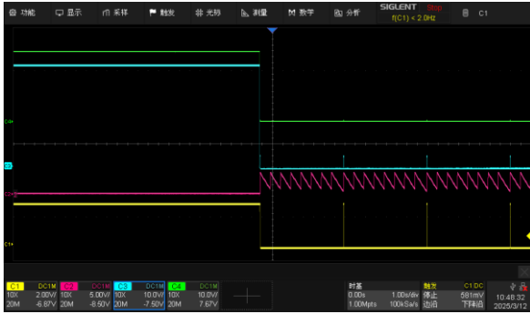
Over current protection
