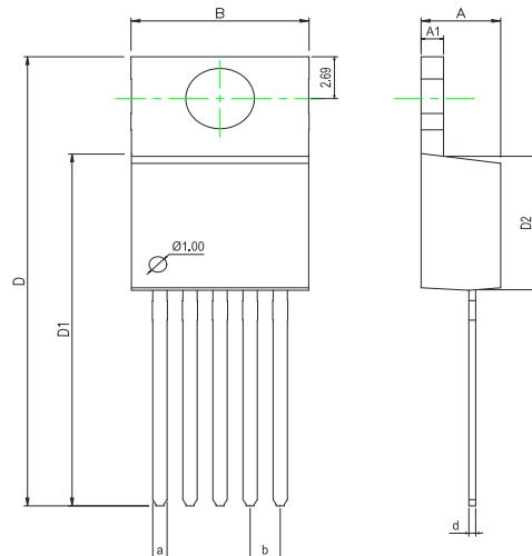
**Dimensions In Millimeters(TO-220-5)**
