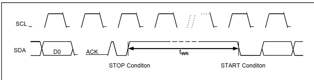
Note: The write cycle time  $t_{WR}$  is the time from a valid stop condition of a write sequence to the end of the internal clear/write cycle.
