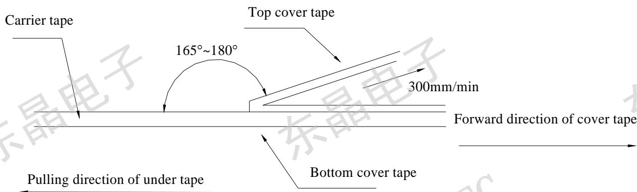
\*\*\* In the case, the cover tape is pulled off under the above conditions the cover tape adhesion strength should be as follows. \*\*\*
