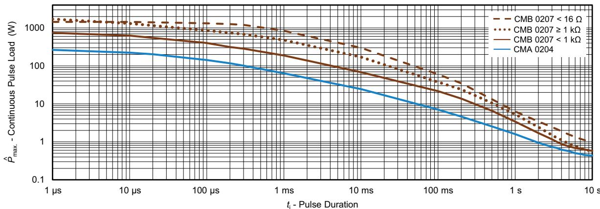
Maximum pulse load, continuous pulse; applicable if  $\bar{P} \leq P(v_{\text{amb}})$  and  $\hat{U} \leq 4$  kV (CMB);
