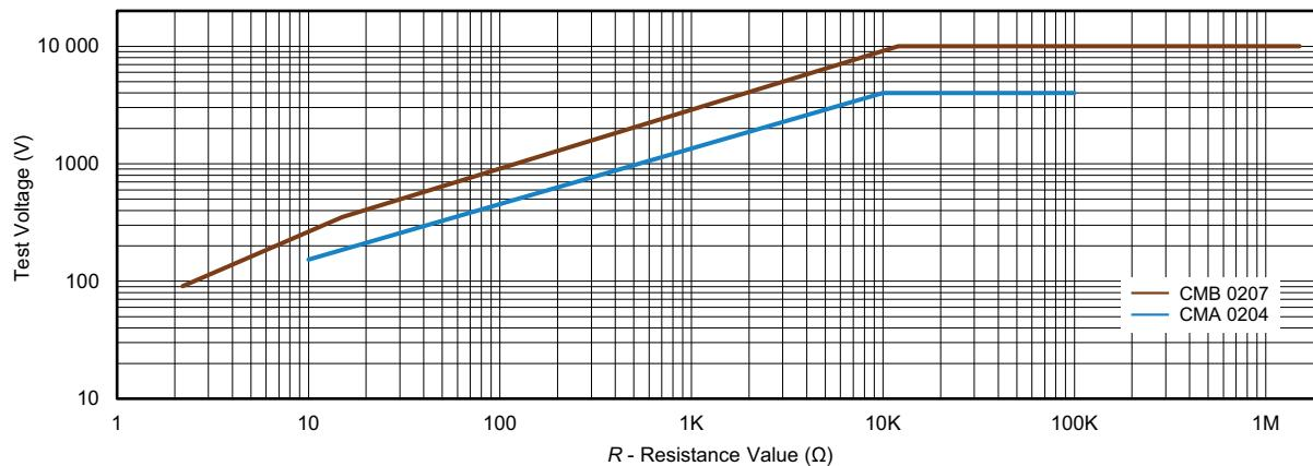
Pulse load rating in accordance with IEC 60115-1, clause 4.27; 1.2 μs / 50 μs; 5 pulses at 12 s intervals;
