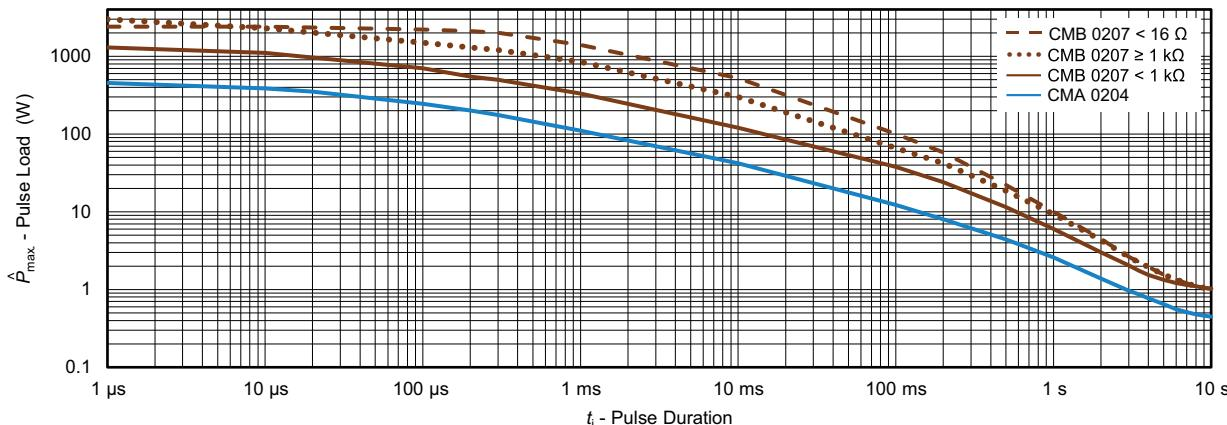
Maximum pulse load, single pulse; applicable if  $\bar{P} \rightarrow 0$  and  $n \leq 1000$  and  $\hat{U} \leq 4$  kV (CMB),
