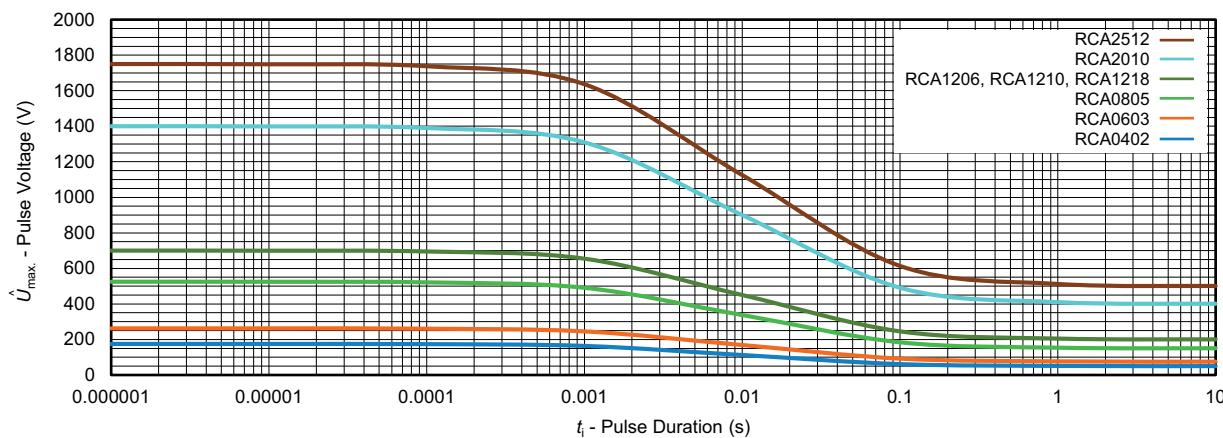
Maximum pulse voltage, single and continuous pulses; applicable if  $\hat{P} = \hat{P}_{\max}$ ;
