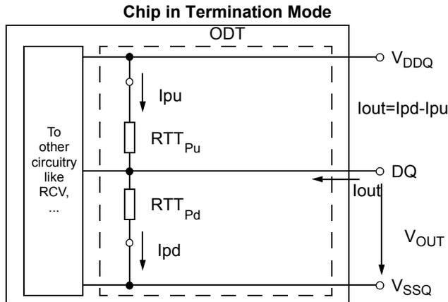
Figure 12. On-Die Termination : Definition of Voltages and Currents
