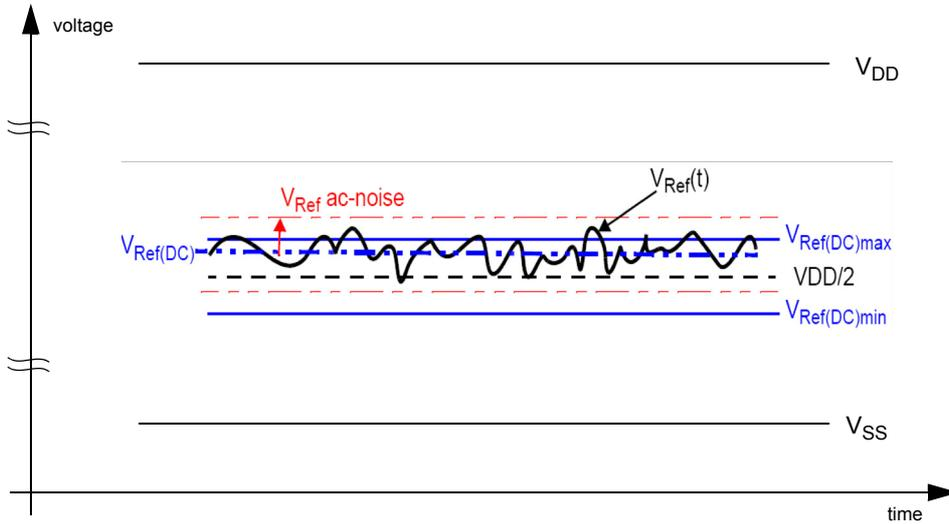
Figure 1. Illustration of V<sub>REF</sub>(DC) tolerance and VREF ac-noise limits
