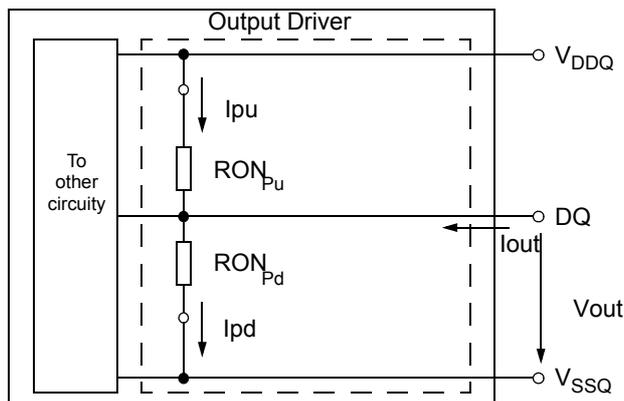
Figure 11. Output Driver : Definition of Voltages and Currents
