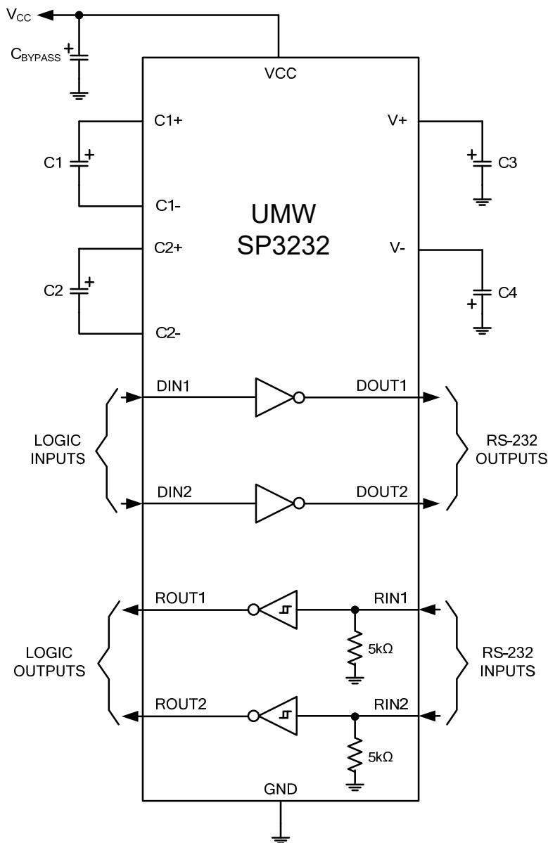
Notes: 1.C3 can be connected to  $V_{CC}$  or GND.
