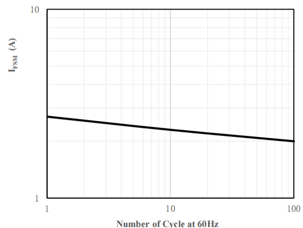
Fig 6 Surge Current Derating Curve
