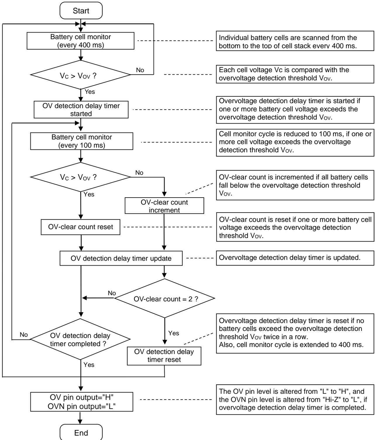
Individual battery cells are scanned from the bottom to the top of cell stack every 400 ms.
