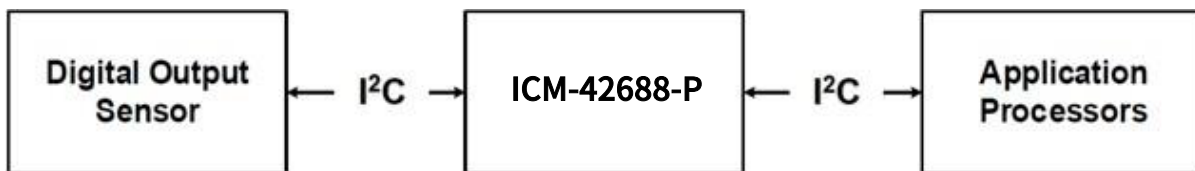
Figure 12: Connection diagram through the auxiliary I 2 C bus
