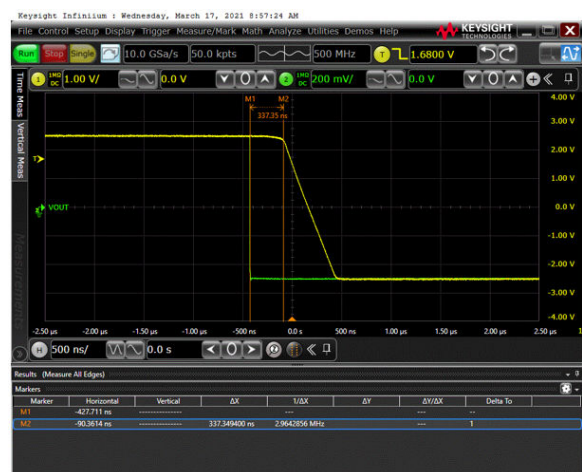
Figure 16. Overload Recovery at Positive Rail
