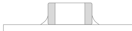
Not enough solder Weak holding force may cause bad connections or detaching of the capacitor
