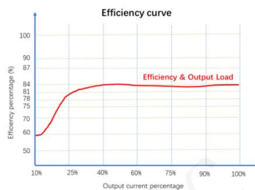
Figure 5: Efficiency VS Output Load (Nominal Voltage Input)
