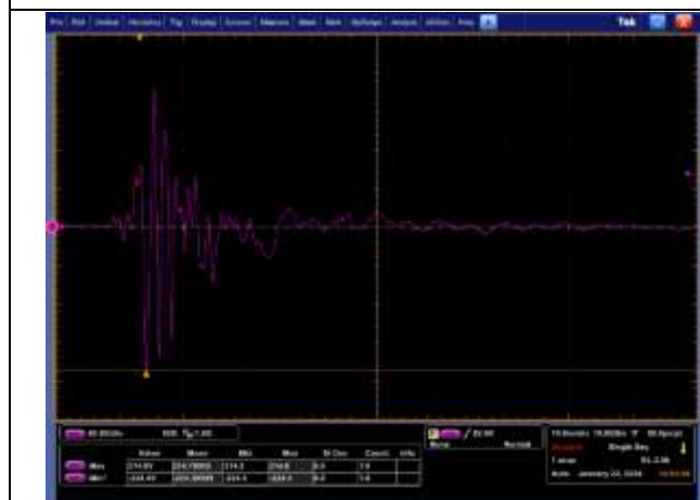
IEC6100-4-2 +8kV IO-IO
