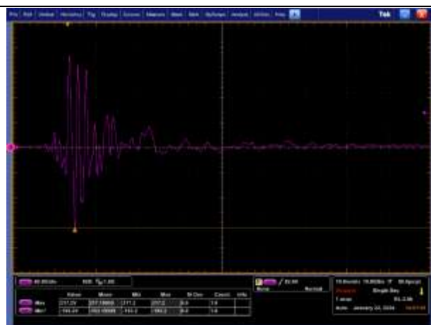
IEC6100-4-2 -8kV IO-IO
