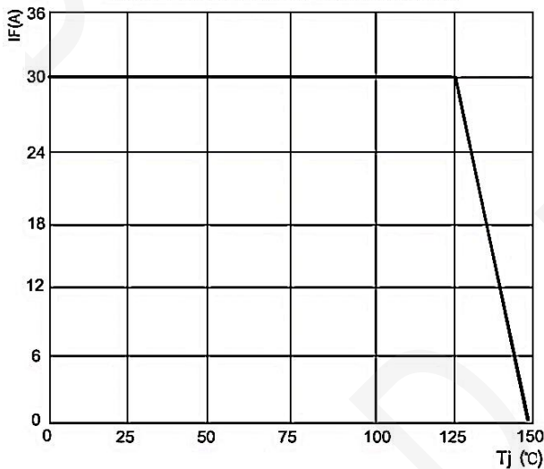
FIG.1: FORWARD CURRENT DERATING CURVE
