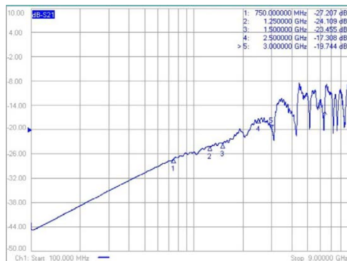
Fig.6 Switch Off Isolation
