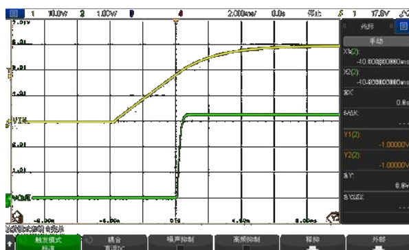
V_{in}=30V, I_{out}=0mA, C_{out}=0.1\mu F
