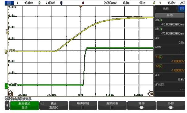
V_{in}=30V, I_{out}=0mA, C_{out}=10\mu F
