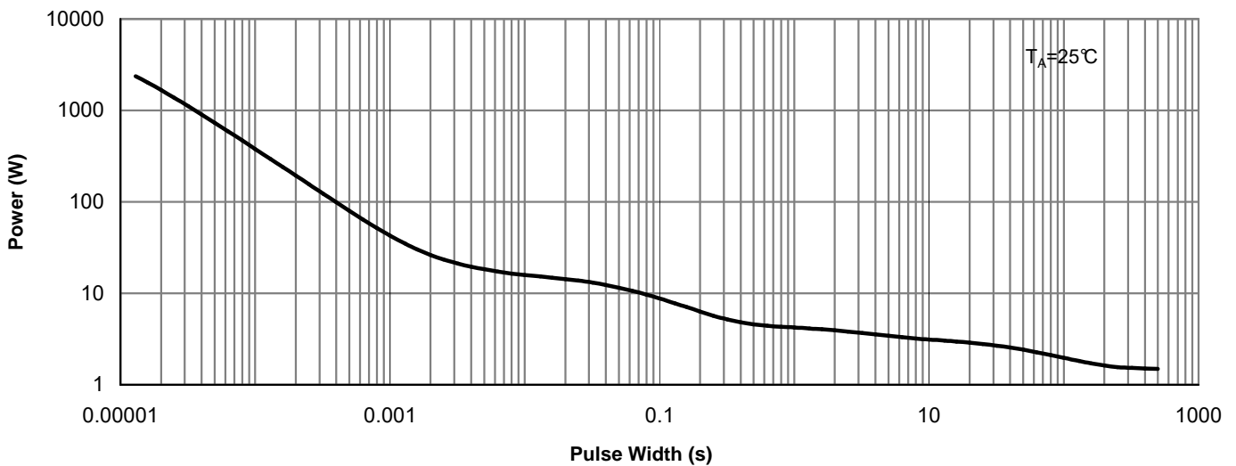
Figure 11: Single Pulse Power Rating Junction-to-Ambient (Note F)
