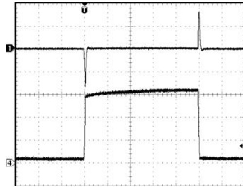
FIGURE 2-28: Line Transient Response with 3A Load, 10 \mu F Output Capacitance.
