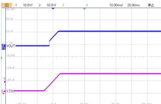
Power-Up at V_{OUT}=12V : ( I_{OUT}=200mA )
