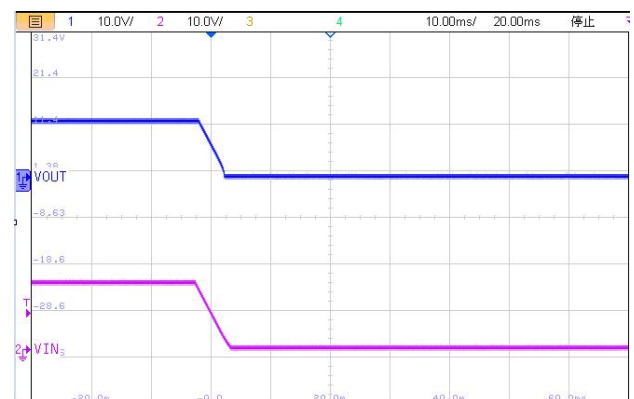
Power-Down at V_{OUT}=12V : ( I_{OUT}=200mA )
