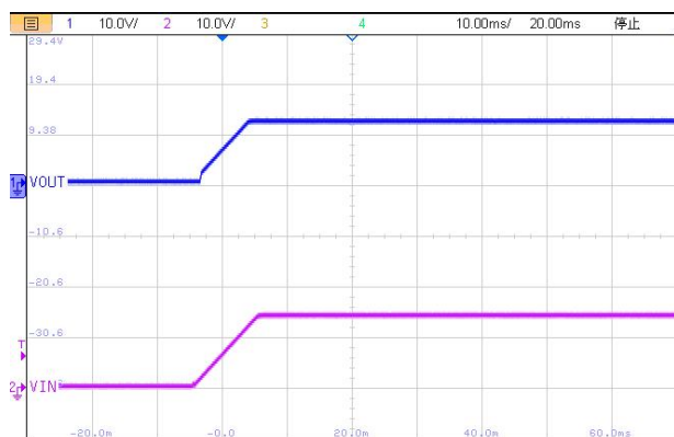
Power-Up at V_{OUT}=12V : ( I_{OUT}=1mA )
