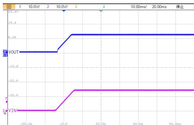
Power-Up at V_{OUT}=12V : ( I_{OUT}=1mA )
