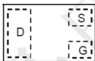
Top View Package Pin Configuration
