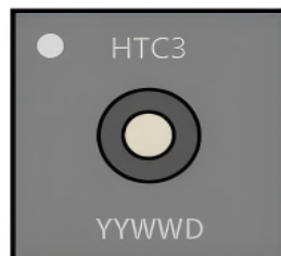
Figure 9. SHTC3-P-NF front laser marking
