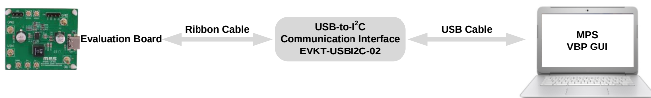
Figure 1: EVKT-MPQ4241 Evaluation Kit Set-Up
