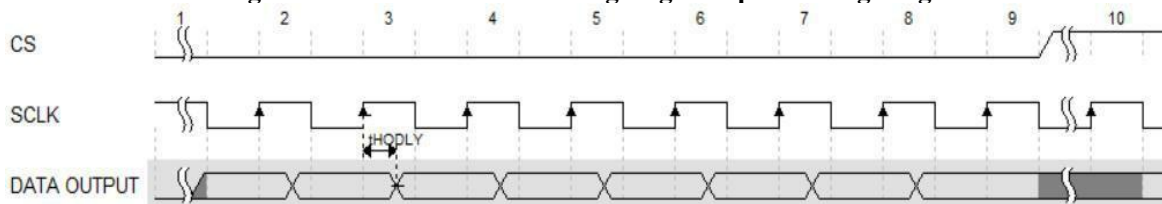
Figure 12-3. HSOD=1 Data Rising Edge Output Timing Diagram
