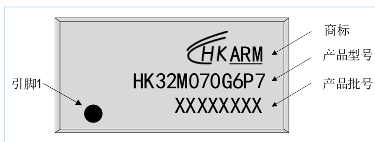
图 7-8 TSSOP28 HK32M070G6P7 丝印示例
