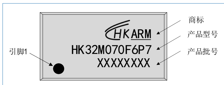
图 7-9 QFN20 HK32M070F6P7 丝印示例
