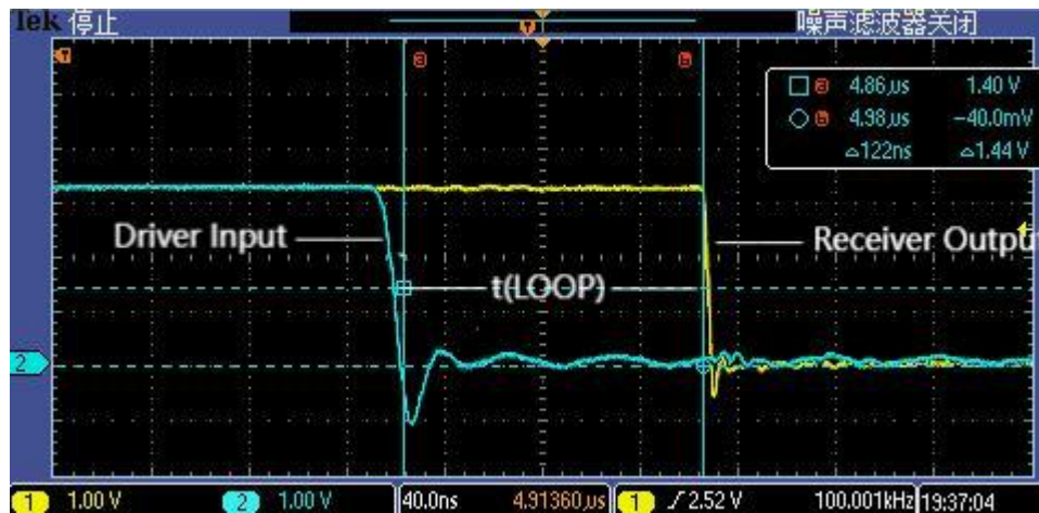
Figure 18. 122-ns Loop Delay Through the SN65HVD230 With R_s = 0
