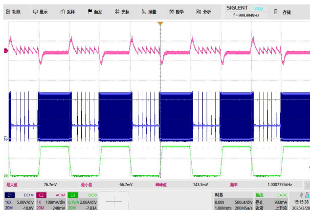
Load Transient VIN=12V, VOUT=3.3V, IO=0A to 3A
