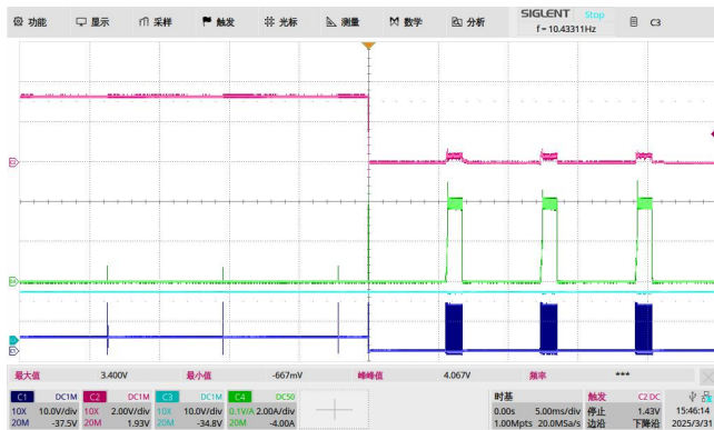
Output Short Entry V_{IN}=12V , V_{OUT}=3.3V , No Load
