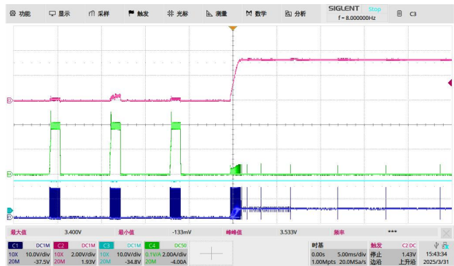
Output Short Recovery V_{IN}=12V , V_{OUT}=3.3V , No Load
