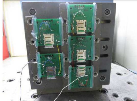
Fig. 6 Set up of Vibration (X axis)
