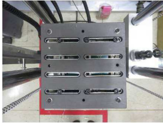
Fig. 11 Set up of Mechanical shock (-Z axis)
