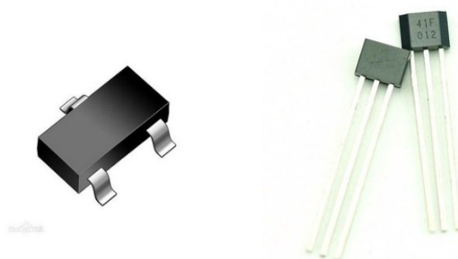
Figure 4: Hall IC (Output Logic Polarity Signal)
