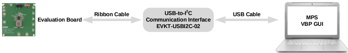
Figure 2: EVKT-MP8880A Evaluation Kit Set-Up
