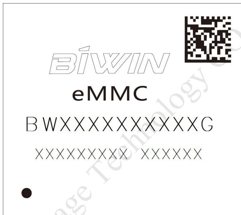
Figure.11 Schematic diagram of product marking
