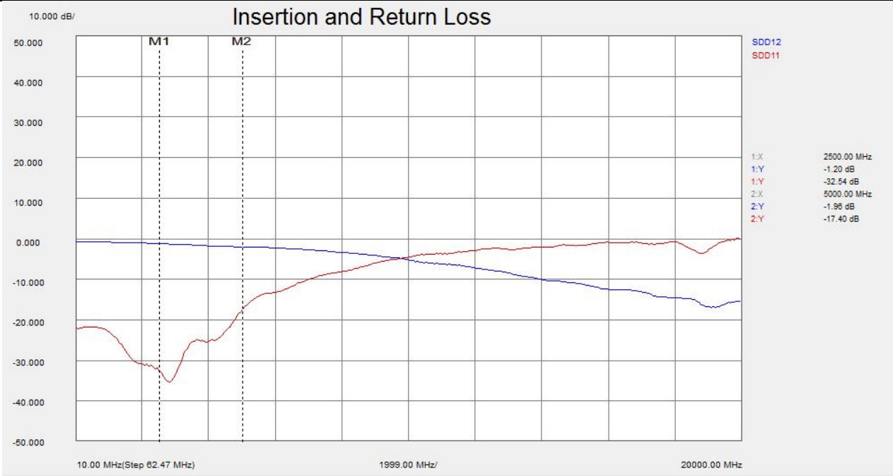
Figure 10: Test Waveform for the Insertion Loss and Return Loss
