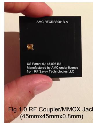
Fig 1.0 RF Coupler/MMCX Jack (45mmx45mmx0.8mm)
