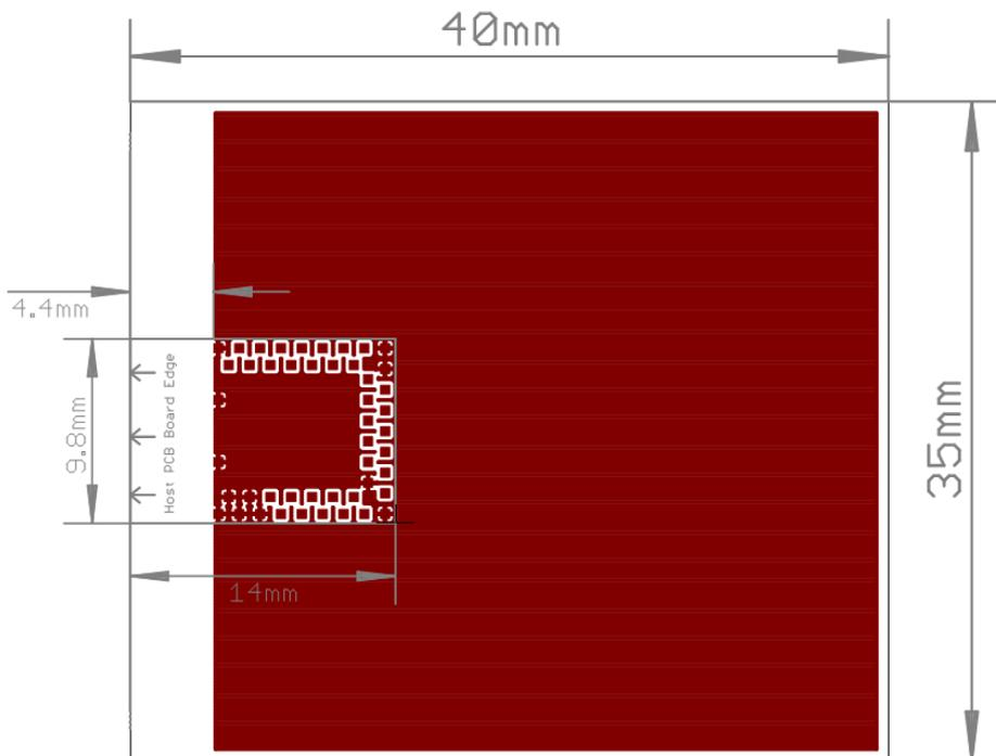
**Figure 8: Recommended RF layout and ground plane for BMD-360**
