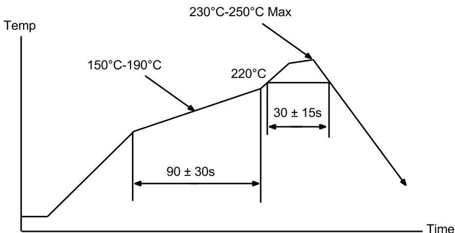
Figure 17: Reflow profile for lead free solder
