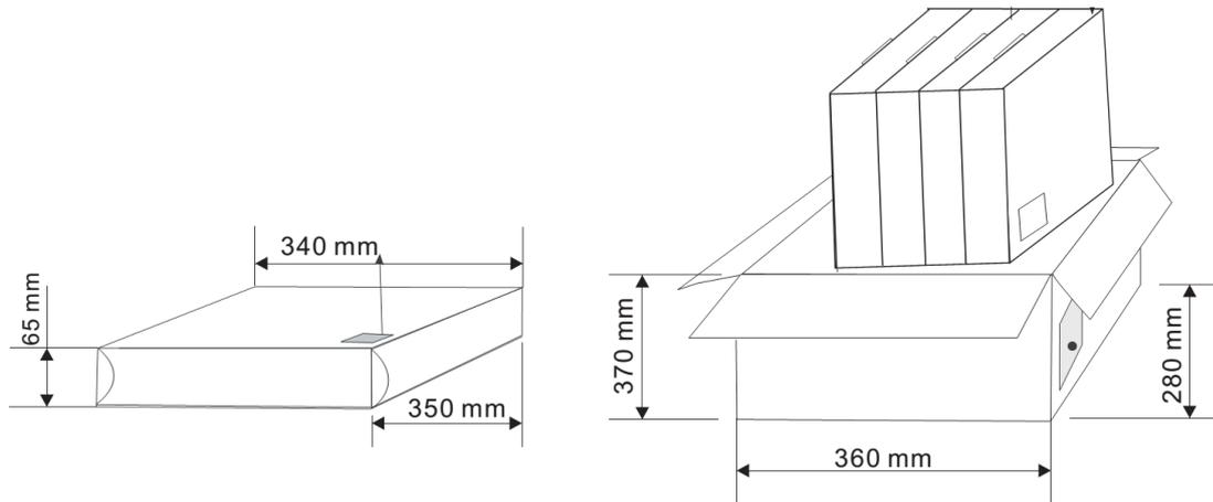
Figure 13: Reel cartons used for type number BMD-360-A-R-00
