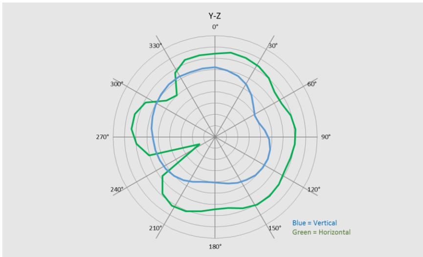
Figure 12: Y-Z Plane Antenna Pattern
