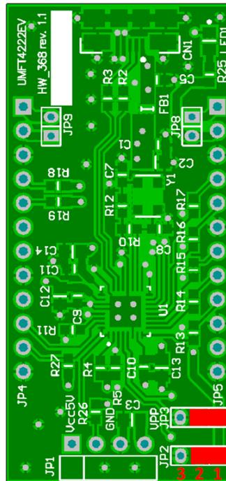
Figure 5-1 JP2/JP3 configuration example: Mode 3 (DCNF0 = 1, DCNF1 = 1)
