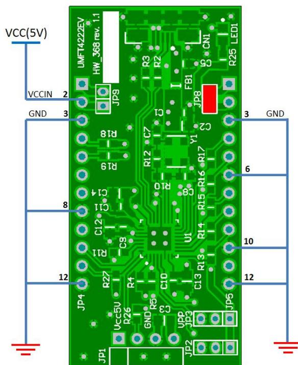
**Figure 7-2 Self-Powered Configuration: Remove Jumper on JP9**
