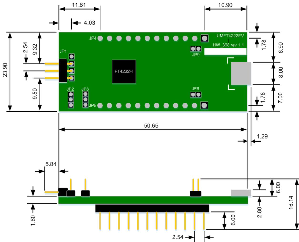
Figure 6-1 UMFT4222EV Module Dimensions
