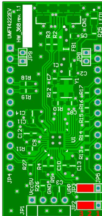
Figure 5-2 JP2/JP3 configuration example: Mode 0 (DCNF0 = 0, DCNF1 = 0)
