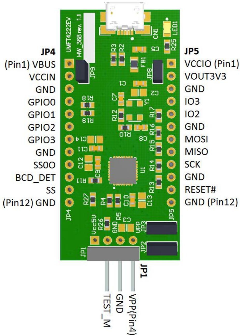
Figure 4-1 Module Pin Out and Jumper Locations
