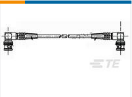
TE Part #1337773-2 50/OHM COAX BNC ELB PLUG ELB P
