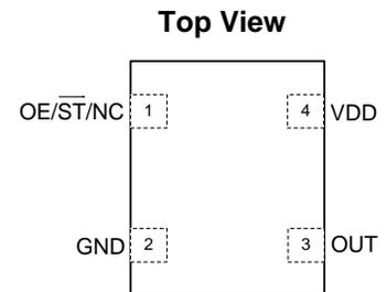
Figure 1. Pin Assignments
