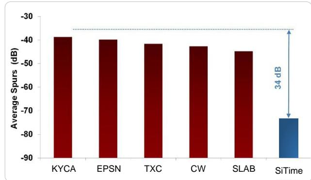
Figure 3. Electro Magnetic Susceptibility (EMS)<sup>[3]</sup>
