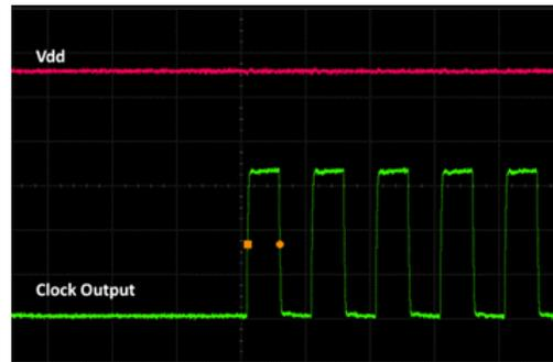
Figure 18. Startup Waveform vs. Vdd
