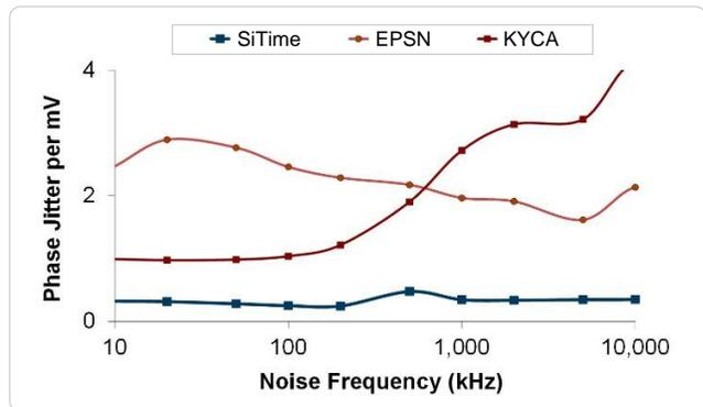
Figure 4. Power Supply Noise Rejection<sup>[4]</sup>
