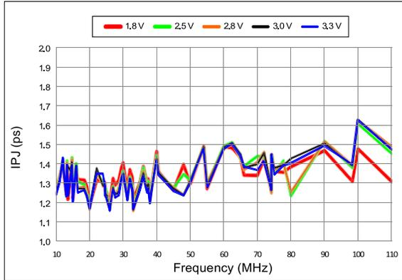
Figure 14. RMS Integrated Phase Jitter Random (12k to 20 MHz) vs Frequency<sup>[9]</sup>
