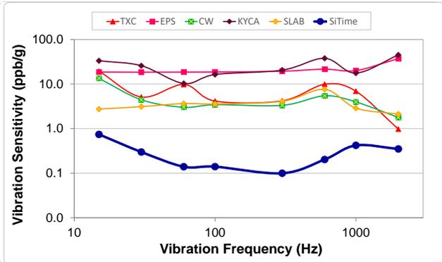
Figure 19. Vibration Robustness<sup>[5]</sup>
