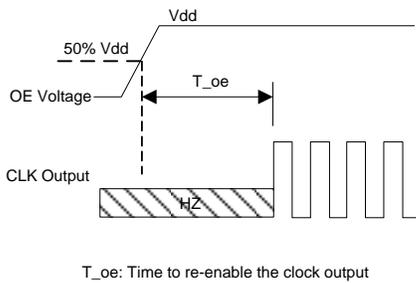
T\_oe: Time to re-enable the clock output
