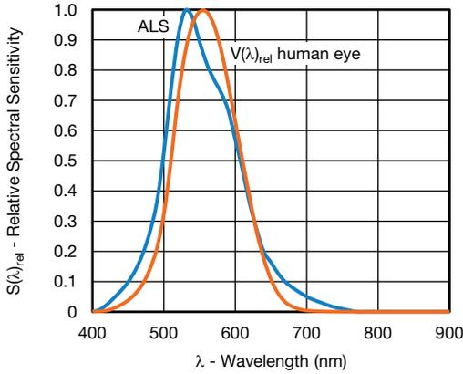
Fig. 5 - Normalized Spectral Response (ALS channel)
