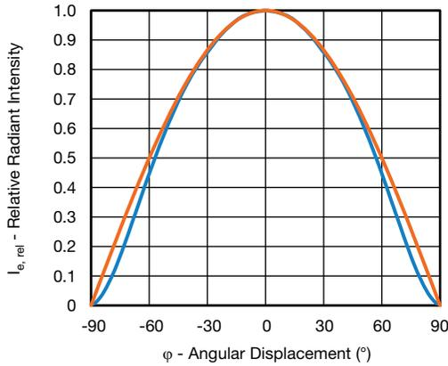
Fig. 11 - Relative Radiant Intensity Emitter vs. Angular Displacement
