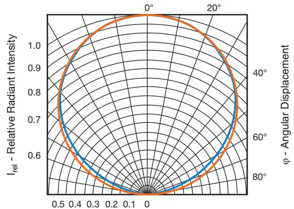
Fig. 10 - Relative Radiant Intensity Emitter vs. Angular Displacement
