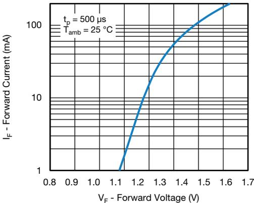
Fig. 7 - Forward Current  $I_F = f(V_F)$  for LED
