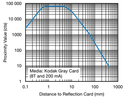
Fig. 15 - Proximity Value vs. Distance to Reflecting Card
