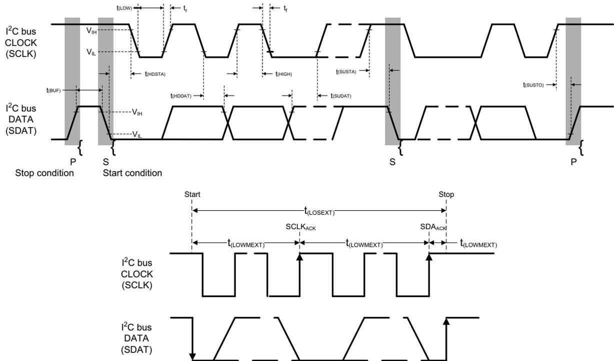
Fig. 2 - I<sup>2</sup>C Bus Timing Diagram
