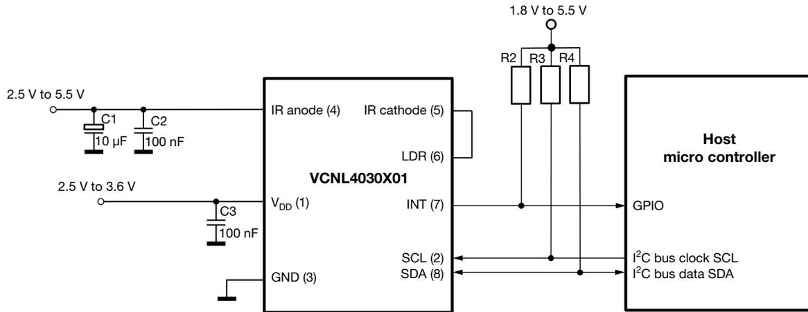
Fig. 16 - Circuitry with Two Separate Power Supply Sources
