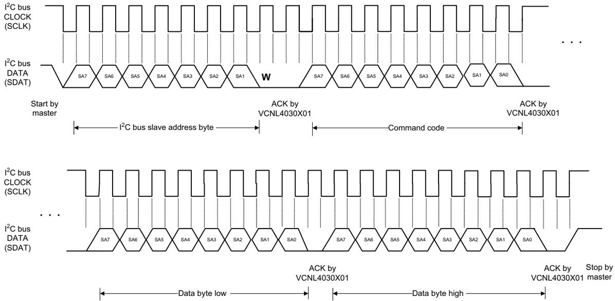
Fig. 3 - I<sup>2</sup>C Bus Timing for Sending Word Command Format
