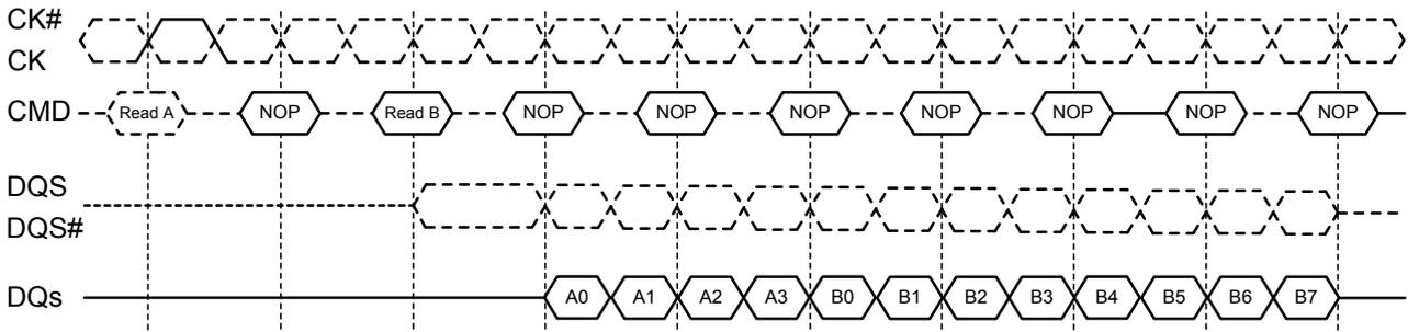
**NOTE 1:** Read burst interrupt function is only allowed on burst of 8. Burst interrupt of 4 is prohibited.
