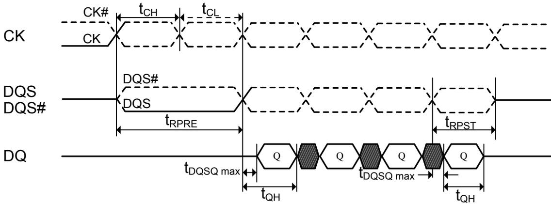
Figure 23. Data input (write) timing
