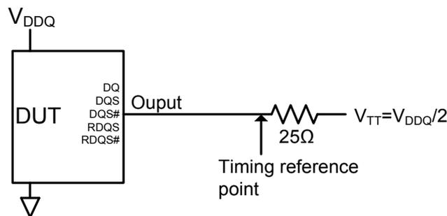
The output timing reference voltage level for single ended signals is the crosspoint with  $V_{TT}$ . The output timing reference voltage level for differential signals is the crosspoint of the true (e.g. DQS) and the complement (e.g. DQS#) signal.
