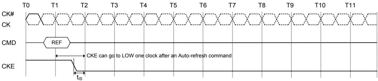
**Figure 58. Active command to power-down entry**
