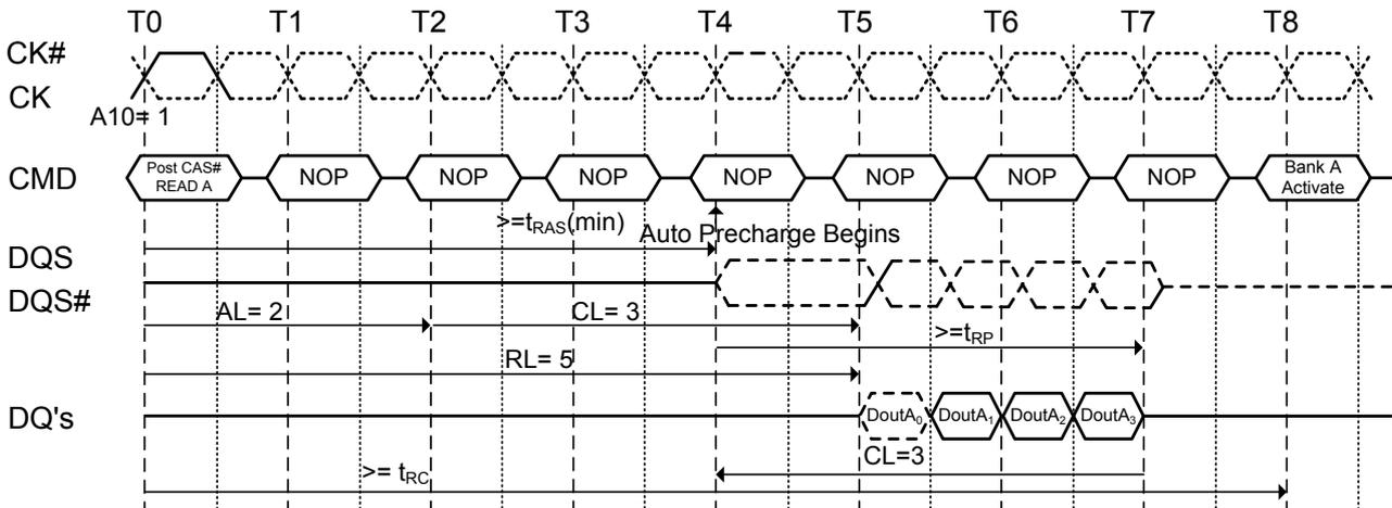
**Figure 45. Burst read operation with auto precharge followed by an activation to the same bank (tRP Limit):**
