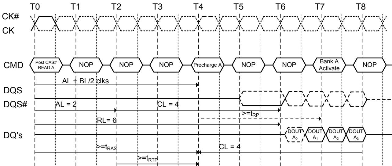
**Figure 39. Burst read operation followed by precharge:**
