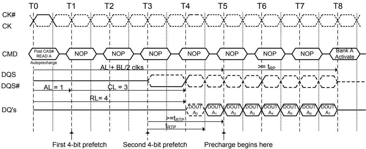
**Figure 43. Burst read operation with auto precharge:
