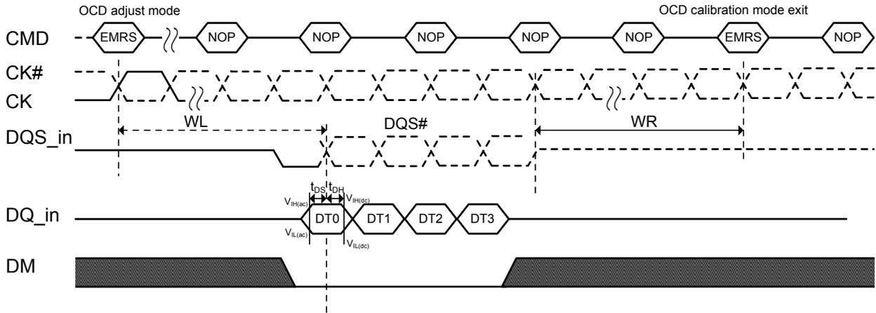
**NOTE 1:** For proper operation of adjust mode,  $WL = RL - 1 = AL + CL - 1t_{CK}$  and  $t_{DS}/t_{DH}$  should be met as shown in the figure.
