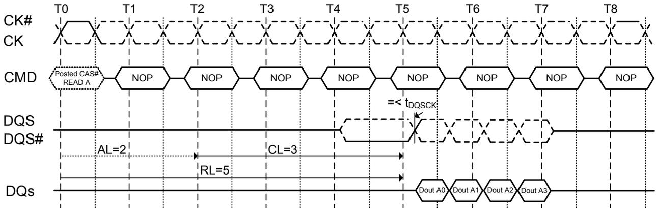
**Figure 25. Burst read operation: RL=3 (AL=0, CL=3, BL=8)**
