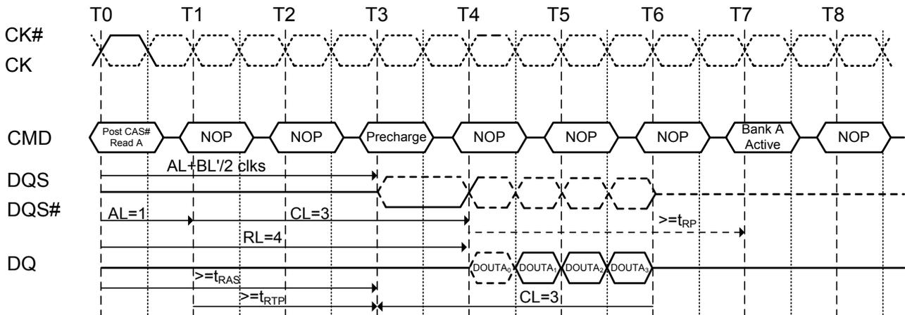
**Figure 36. Burst read operation followed by precharge:**
