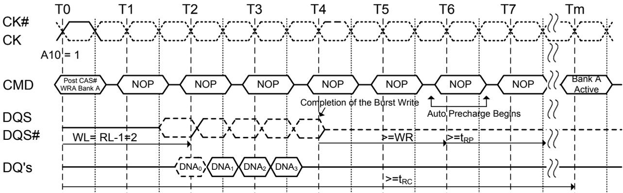
**Figure 47. Burst write with auto-precharge (WR+t<sub>RP</sub>): WL=4, WR=2, BL=4, t<sub>RP</sub>=3**
