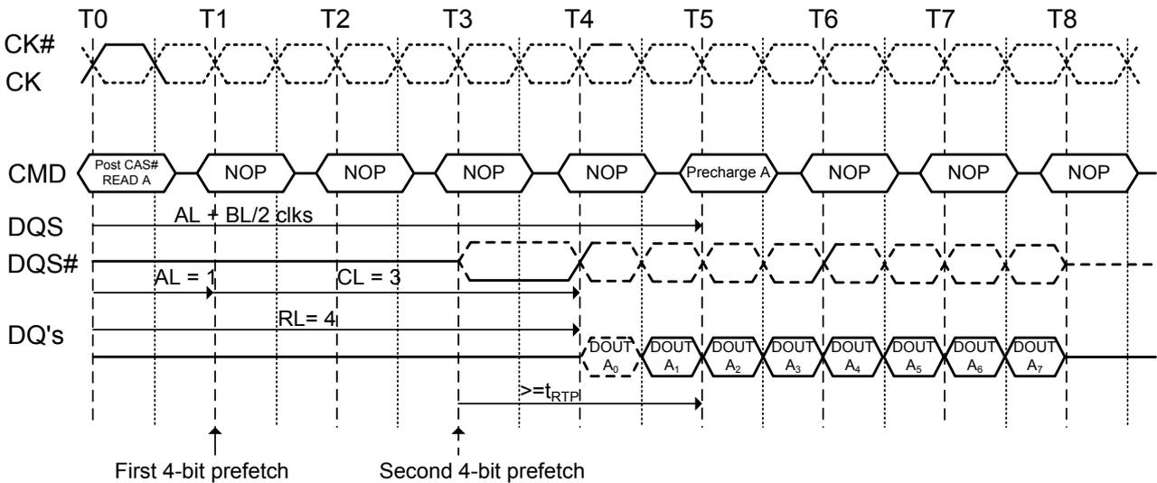
**Figure 37. Burst read operation followed by precharge:**
