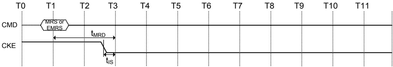
**Figure 61. Asynchronous CKE LOW event**
