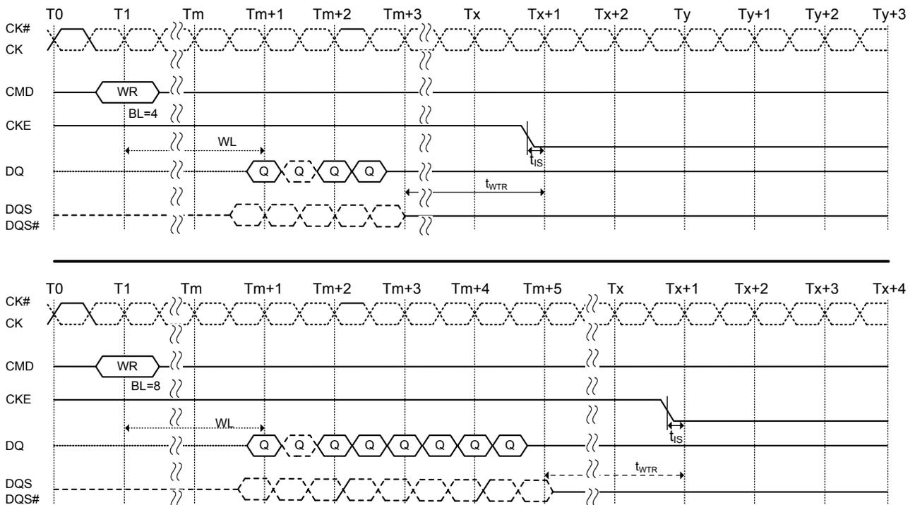
**Figure 56. Write with autoprecharge to power-down entry**
