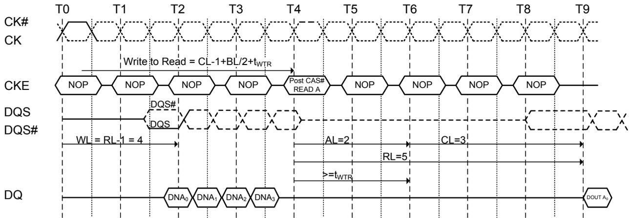
**NOTE :** The minimum number of clock from the burst write command to the burst read command is  $[CL-1 + BL/2 + t_{WTR}]$ . This  $t_{WTR}$  is not a write recovery time ( $t_{WR}$ ) but the time required to transfer the 4 bit write data from the input buffer into sense amplifiers in the array.  $t_{WTR}$  is defined in the timing parameter table of this standard.
