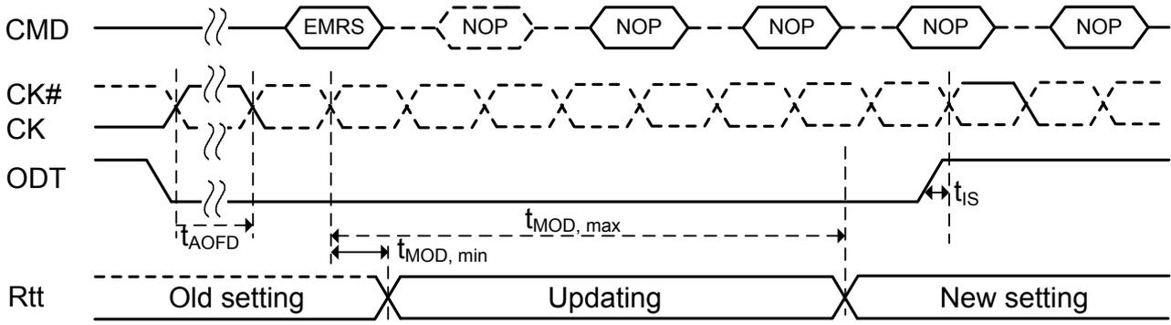
**NOTE 1:** To prevent any impedance glitch on the channel, the following conditions must be met:
