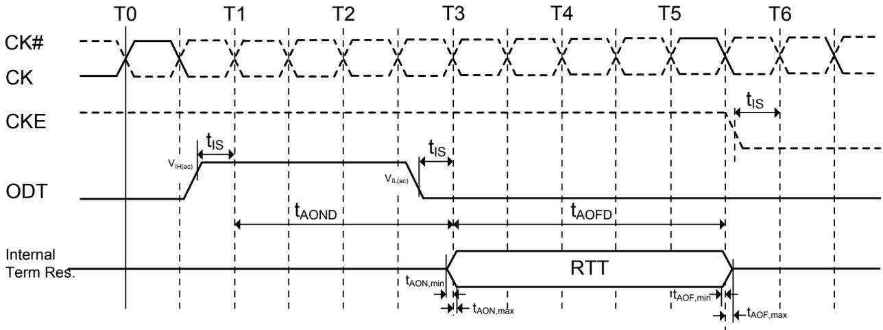
Figure 16. ODT timing for power-down mode
