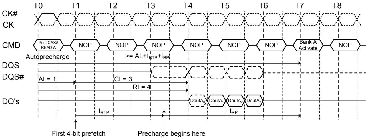
**Figure 44. Burst read operation with auto precharge followed by activation to the same bank ( $t_{RC}$  Limit):
