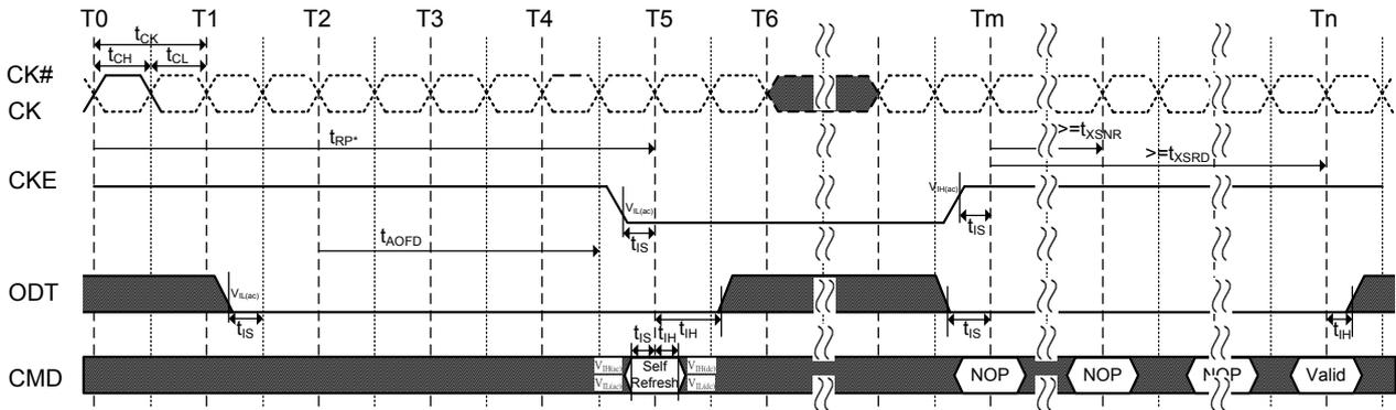
NOTE 1 Device must be in the "All banks idle" state prior to entering Self Refresh mode.
