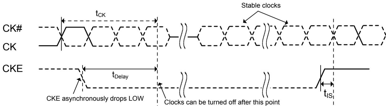
**Figure 62. Clock frequency change in precharge power down mode**
