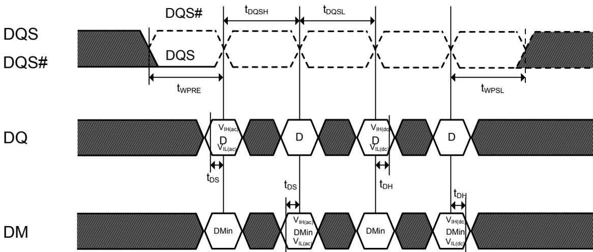
**Figure 24. Burst read operation: RL=5 (AL=2, CL=3, BL=4)**
