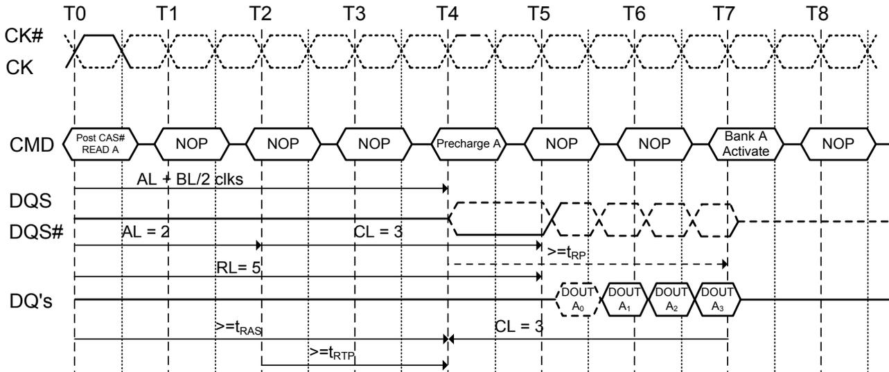
**Figure 38. Burst read operation followed by precharge:**
