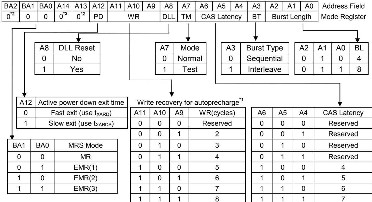
Note 1. For DDR2-800, WR min is determined by  $t_{CK} (avg)$  max and WR max is determined by  $t_{CK}(avg)$  min.  $WR [cycles] = RU \{t_{WR}[ns]/t_{CK}(avg)[ns]\}$ , where RU stands for round up. The mode register must be programmed to this value. This is also used with  $t_{RP}$  to determine  $t_{DAL}$ .
