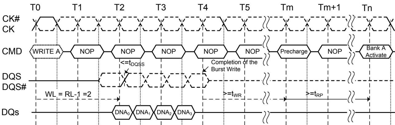
**Figure 31. Burst write followed by burst read:
