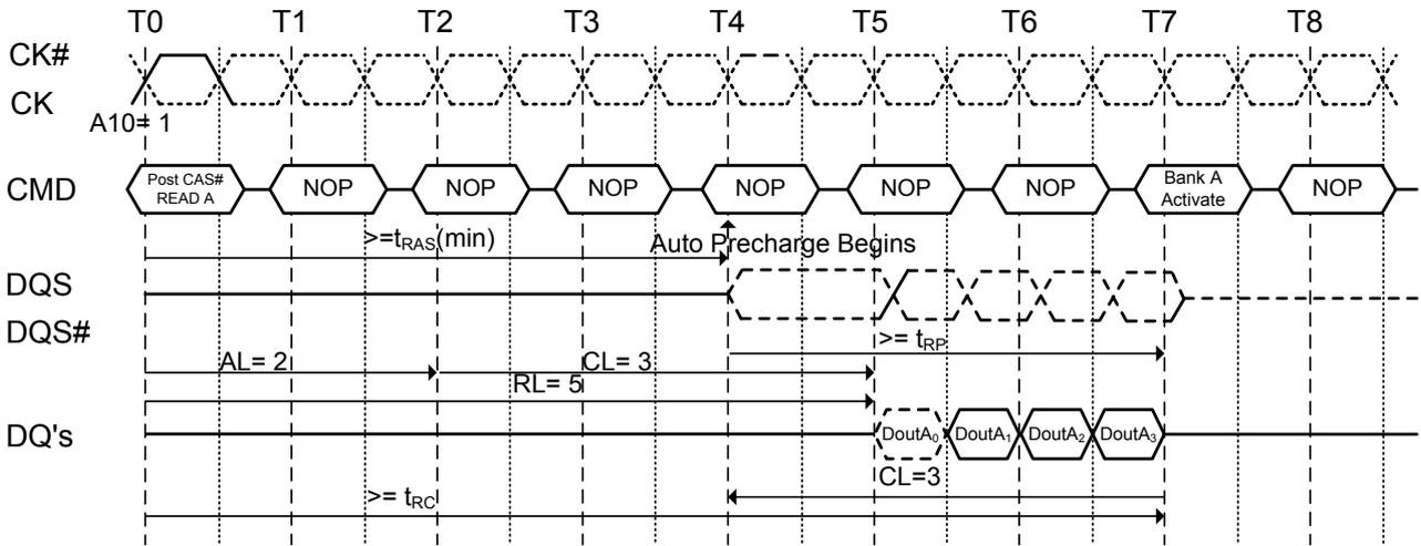
**Figure 46. Burst write with auto-precharge (t<sub>RC</sub> Limit): WL=2, WR=2, BL=4, t<sub>RP</sub>=3**
